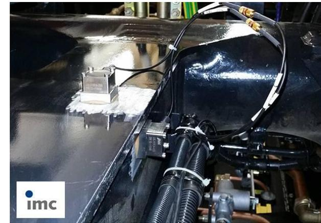
Acceptance tests of a new long-distance train, measuring specialist imc utilized ASC sensors
